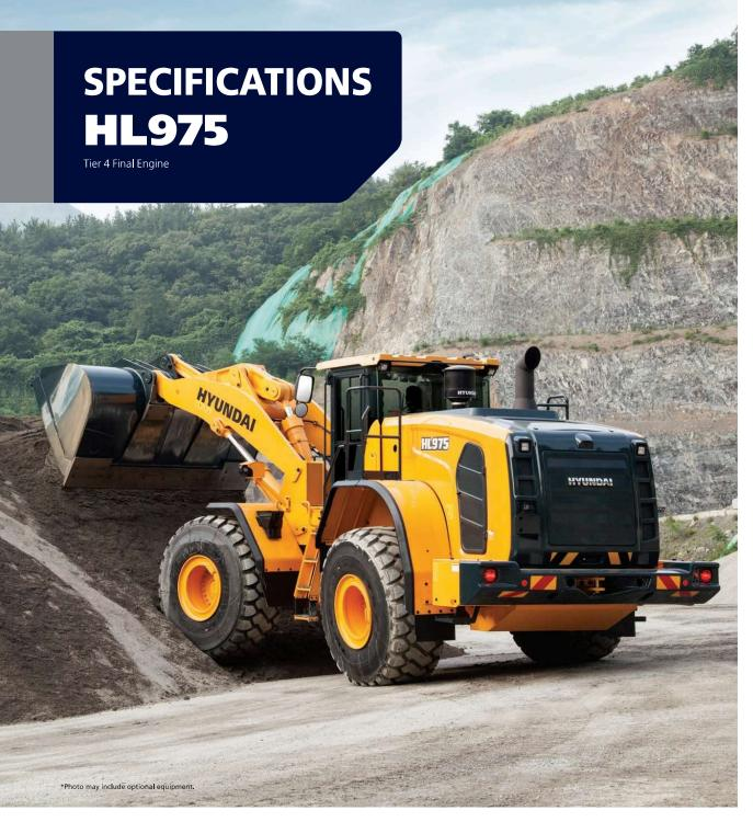
331 HP (247 kW)/2,100 rpm | 26,500 kg/58,430 lb | 4.8 m³/6.3 yd³
