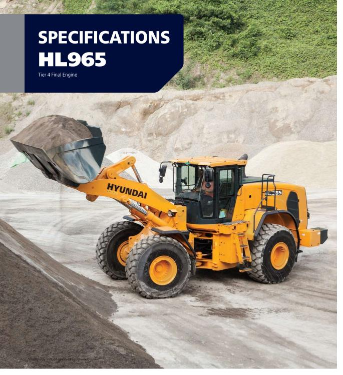
269 HP (198 kW)/2,100 rpm | 20,730 kg/45,700 lb | 3.6 m<sup>3</sup>/4.7 yd<sup>3</sup>
