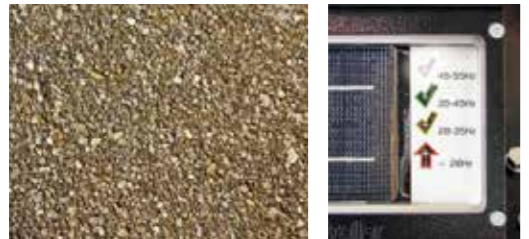
Non-binding soil (sand, gravel); High frequency approx. 45-55 Hz
