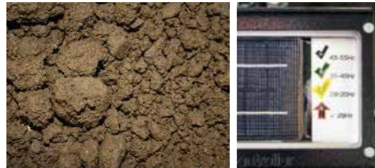
Tied floors (clays, silts); Low frequency approx. 28-35 Hz
