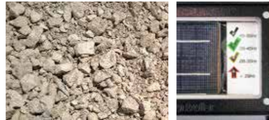
Mixed grained soils; Medium frequency approx. 35-45 Hz; UNIVERSAL FREQUENCY
